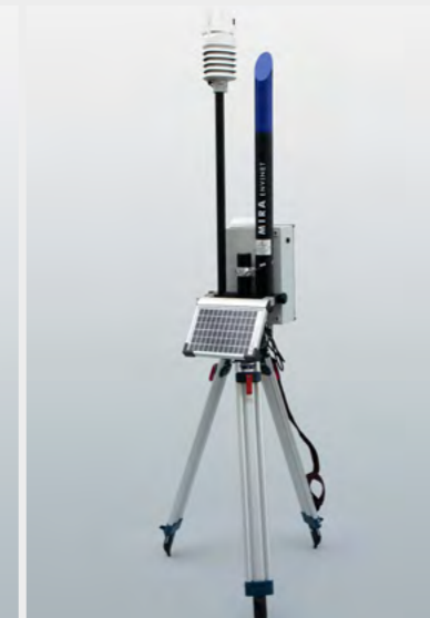
Gamma & Weather Monitoring Station
